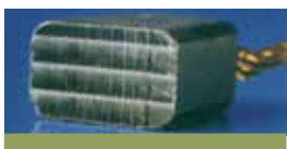
S17 ■ Lamination of sliding face
