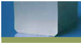
S1 ■ Dense, shining sliding face
