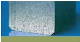
S3 ■ Slight porous sliding face
