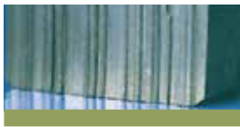
S9 ■ Tracking with hairlining and groves
