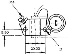
Complete with an *'RS70'* Silver Graphite Brush – 6.4mm x 10 x 23mm long The maximum space required for fitting is 55mm x 35mm x 20mm The mounting holes are pre-threaded to accept M4 screws
